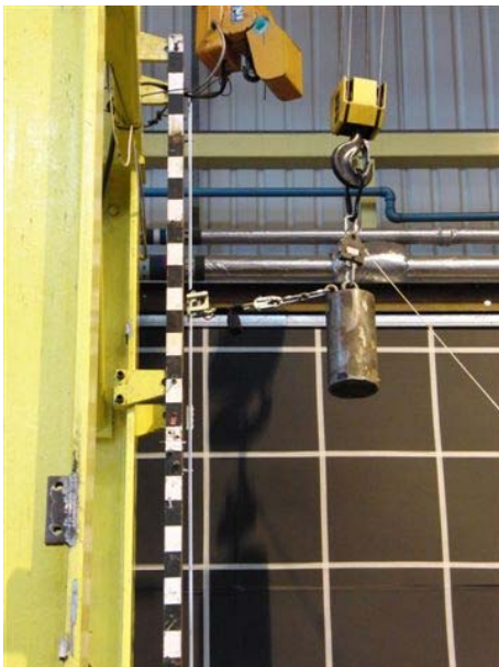
Figure 3 Dmax Test Set-up Test mass positioned 455 mm from the system rail.
